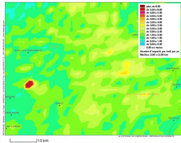
Fig. 2. Ground flash density in the experiment area
