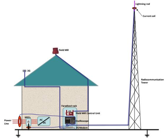
Fig. 1. Functionnal diagram of the experiment
